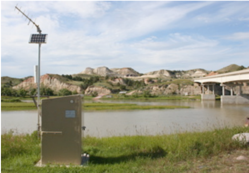
Modern U.S. Geological Survey Stream Gauge at the Culbertson Bridge, Montana.
